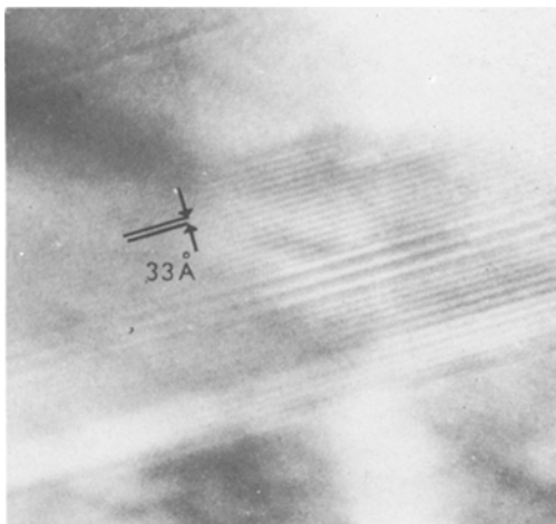
Figure 6 33 Å spacing typical of the three-block \beta'' structure.
